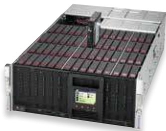
4U Storage 60x 3.5" SAS3 Drive Bays, w/ IT mode controller, Storage Expandable
