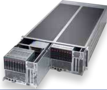
FatTwin™ 2 DP Nodes, 6 GPU/Coprocessor per Node, Front I/O, 16 DIMMs
