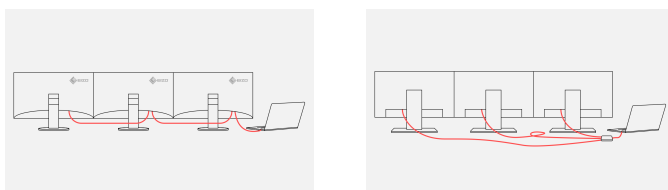
Daisy chain method Tidied-up cables
